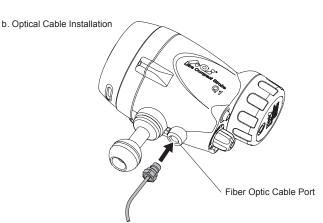
Plug the Optical Cable into Q1 Fiber Optic Cable Port and the other end to the camera housing
