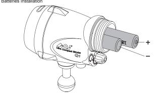
To install the batteries, take off the Battery Cap and put in the batteries with the correct polarity as indicated in the battery chamber. - 3 -
