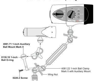
Mounts to the Auxiliary Ball Clamp for the attachment of additional lightweight accessories in the middle of your strobe arm. Requires the 4081.22 1-inch Ball Clamp Mark II with Auxiliary Mount, sold separately. Using a flathead screwdriver, tighten the Ball Mount to the Auxiliary Ball Mount Clamp as shown. **Note:** Ball components with an o-ring groove should have an o-ring installed at all times.
