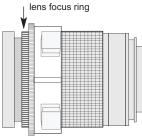
4. Insert camera lens through front port opening and align with lens mounting indicator on the camera body. Rotate lens clockwise until lens locks into place.
