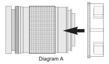
3 Slide the Zoom Sleeve forward until the front edge aligns with the focus ring of the camera lens.
