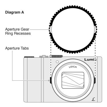
**3.** Press Gear Ring over Aperture Tabs.
