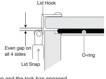
5. Check the o-ring seal. The o-ring should form a solid uniform line around the back of the housing, denoting a good seal. There will be a small even gap around the housing between the housing back and front.
