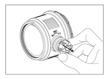
Make sure the control knob is at its most outwards position before mounting/ unmounting the port. The knob should be left at this position until it is made sure that the lens and focus/zoom gear is properly installed.
