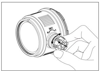
2. Engage the gear by pushing in the knob, then turn the knob both ways to check if the lens focuses/zooms.
