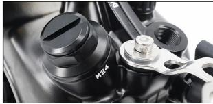
Place the M24-M16 Step Down Adaptor on the M24 accessory port opening, then fasten the adaptor.
