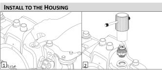
Remove the plug of the M14 accessory port from the housing. Remove the cap from the vacuum valve. Tighten the vacuum valve to the housing with the tool provided.
