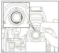
Remove the retainer O-ring of the 0.66x viewfinder inside the rear half of the housing.
