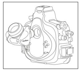
Align the 45° viewfinder with the viewfinder mounting ring in the display window as shown in the diagram.
